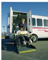
5. ADA Minibus Capacity 10-26 Passengers Typically 15 or 24 Passengers with 1 or 2 Secure Wheelchair Positions
