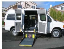
4. Wheelchair Van 1-9 Passenger Typically 2 Secure Wheelchair Positions and 2-3 Ambulatory Seats
