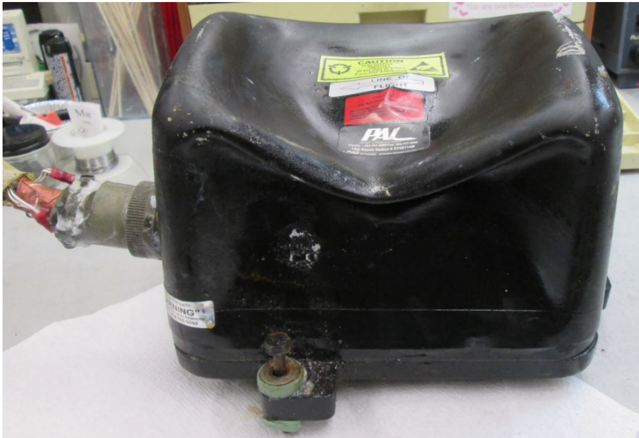
Figure 6. View of inward crushing on the vertical gyro housing.
